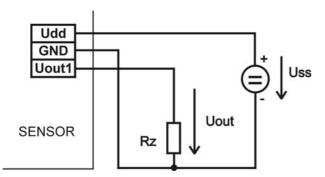
Maximum load current of each voltage output is 0.5 mA
